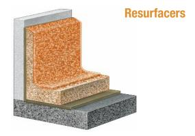
Clear or pigmented epoxy, acrylic or urethane binders fuse with multi-colored or natural quartz aggregate to create a monolithic matrix layer with high tensile strength and superior longevity.
